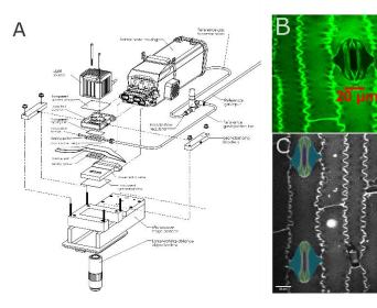
A customized tool to simultaneously measure stomatal aperture and stomatal conductance.
