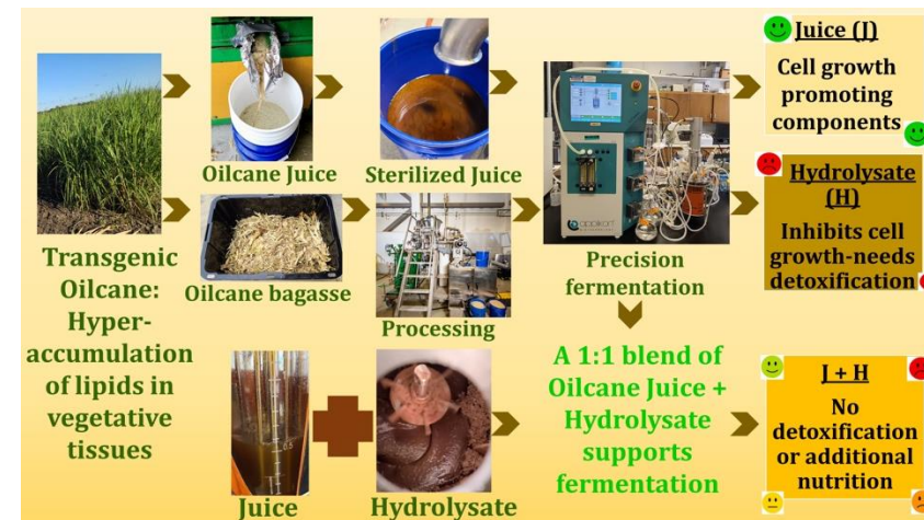
Process diagram of fermentation using equal blends of OC hydrolysate and juice.
