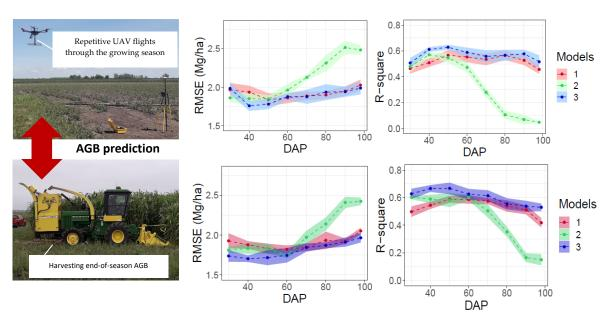
Evaluation of AGB prediction in testing data for timepoint (models 1), dynamic (2), and time-point and dynamic variables (3) via RMSE and R<sup>2</sup> for full (upper panels) flights (n=10), and for reduced (lower panels) flights (n=5).
