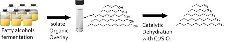
Overview of the integrated process components (biological and catalytic) starting from anerobic fatty alcohol production, going to organic overlay isolation, and finishing with catalytic dehydration to LAO.
